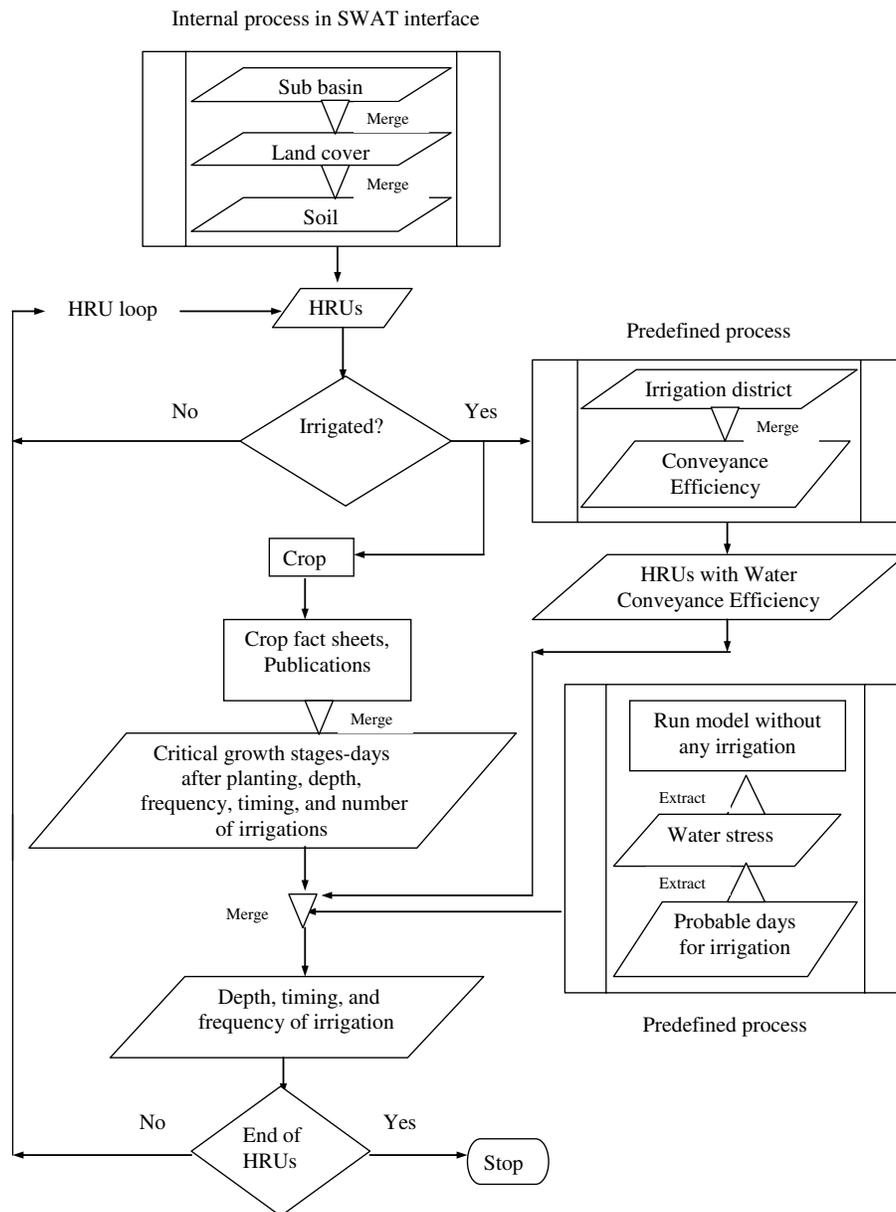
**Fig. 3.** Modeling canal irrigation in the watershed model setup
