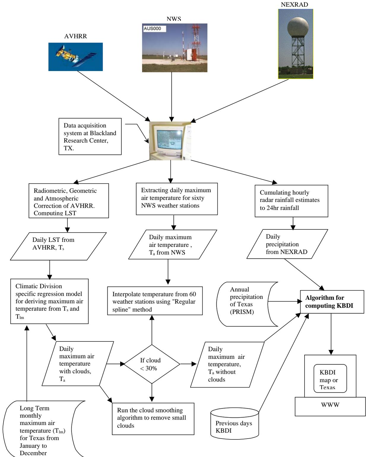
Figure 4. A real-time system for computing KBDI using remotely sensed data and GIS.
